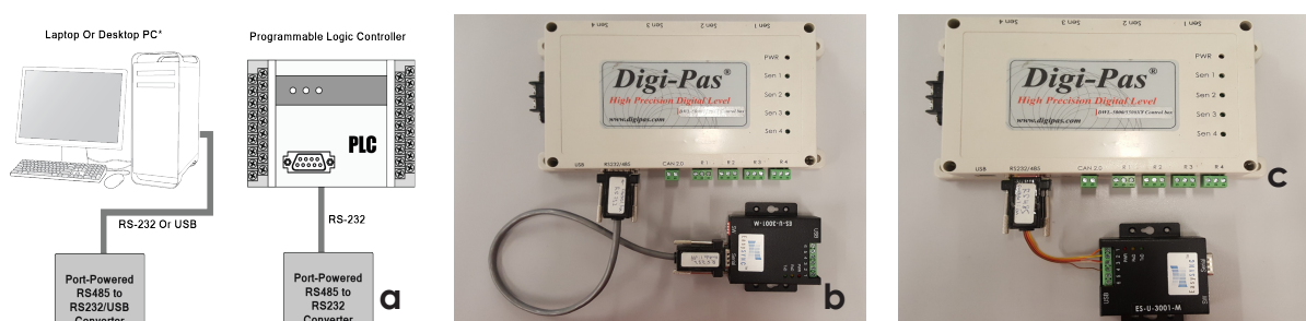
Figure 13. Connection of the control box in (a) USB mode (b) RS232 mode (c) RS485 mode
